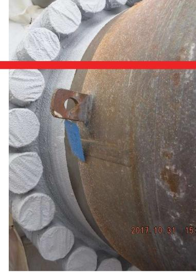
Belzona 3412 was then mixed and applied using a cartridge spray gun over most of the surface and with a short bristle brush over hard to reach areas. Two coats of dissimilar colors of Belzona 3412 were applied.
